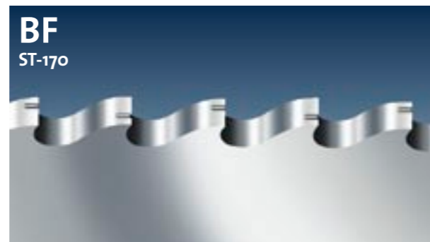
BF ST-170 SHAPE BF: Teeth identical to Shape B, but equipped with chip-breaking features, making it possible to cut the chip into 3 sections of equal width. For cutting tubes with sections under 4 mm. Employed with series 170 for excellent results in high-speed tube cutting.
