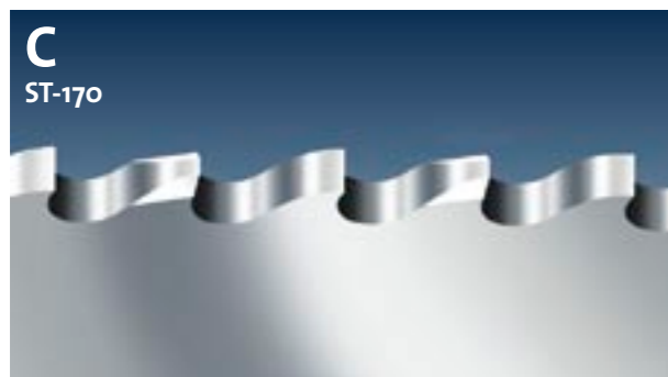
C ST-170 SHAPE C: Alternately high and low teeth, used for cutting large sections. For pitches of over 5 mm with high and low teeth, used in the cutting of large sections. The high teeth are bevelled with chip-breaking features.
