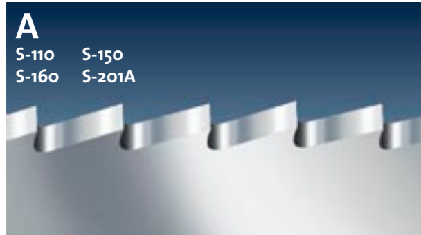
AW SHAPE AW: Small-pitch teeth, used mainly in fine machining tasks. Employed with series 110 and series ST-170 cut-off machines for high-speed cutting of brass. Teeth are bevelled with chip-breaking features.
